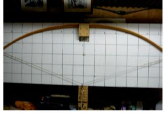
Tillering rig with bow at full draw. To plot your graph, write the poundage at every 2in increment.
