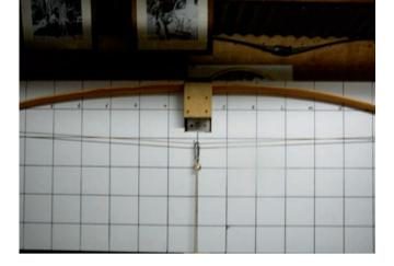
Tillering rig with bow at rest.
