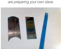
Scrapers of various shapes. A hacksaw blade back will suffice as a scraper.
