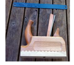
Toothing plane; The plane iron is serrated to achieve a good gluing surface. A coarse hacksaw blade will suffice.
