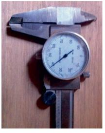
A vernier caliper marked in thousandths of an inch will be valuable if making up your own staves.
